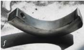
(f) finished hinge stop with threaded hole (g) Russ's diagram of the hinge stop's range of motion on the press (h) hinge stop on the press with the tympan raised, bolt resting against the underside of the corner iron to prevent further rotation
