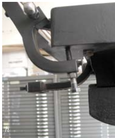
(f) finished hinge stop with threaded hole (g) Russ's diagram of the hinge stop's range of motion on the press (h) hinge stop on the press with the tympan raised, bolt resting against the underside of the corner iron to prevent further rotation
